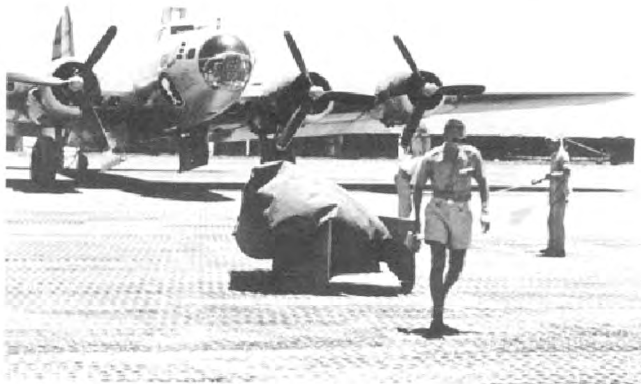
Figure 18. Air sampling gas bag and drone B-17 at Enewetak Island following shot ABLE, CROSSROADS.
